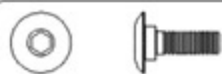
Socket button head collar screw 半圓頭內六角軸套螺絲(M3x8mm) x 2
